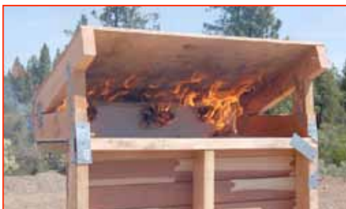
Debris on the outside can lead to flames on the inside!
